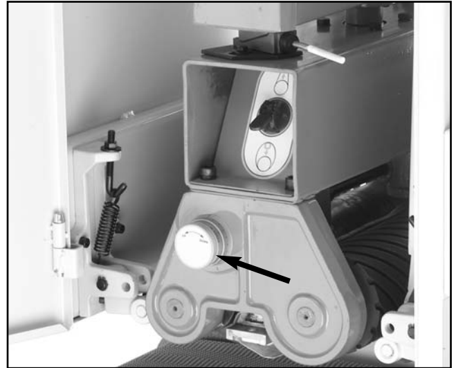
Figure 9. Use this knob to raise/lower the platen.
